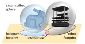
Fig. 4: **Interactions with holograms.** When approaching the hologram, the robot can manipulate a hologram and carry it together if there exists an intersection between their footprints, which triggers the interaction into a manipulation mode.
